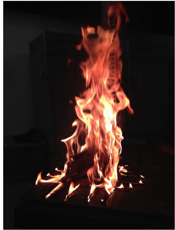
Figure 1. Laboratory burn demonstrating the flame heights of American chestnut ( Castanea dentata ). The average maximum flame height for all observations was 98.9 cm (range = 91–106 cm).
