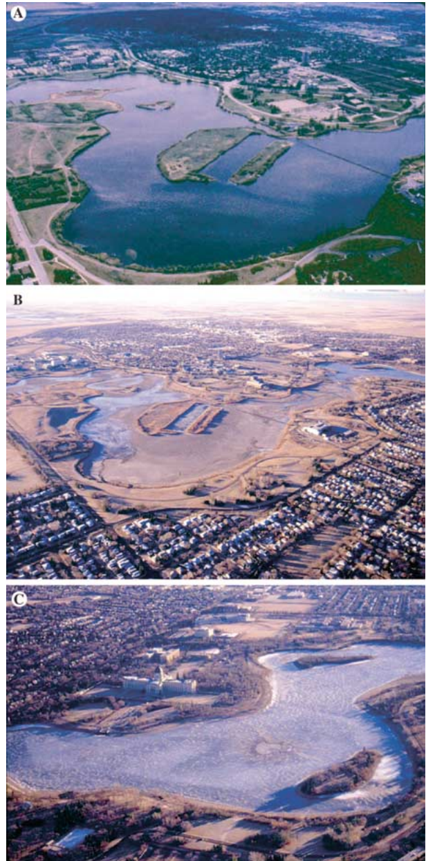
Figure 2. Aerial view of Wascana Lake before (A) and during (B, C) experimental drawdown. Dewatering reduced lake levels approximately 1 m (50% of Z_{\max} ) in the deepest portion of the basin (C).
