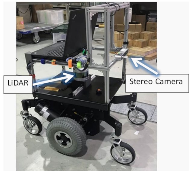
Fig. 11 A mobile robot used in our experiments
