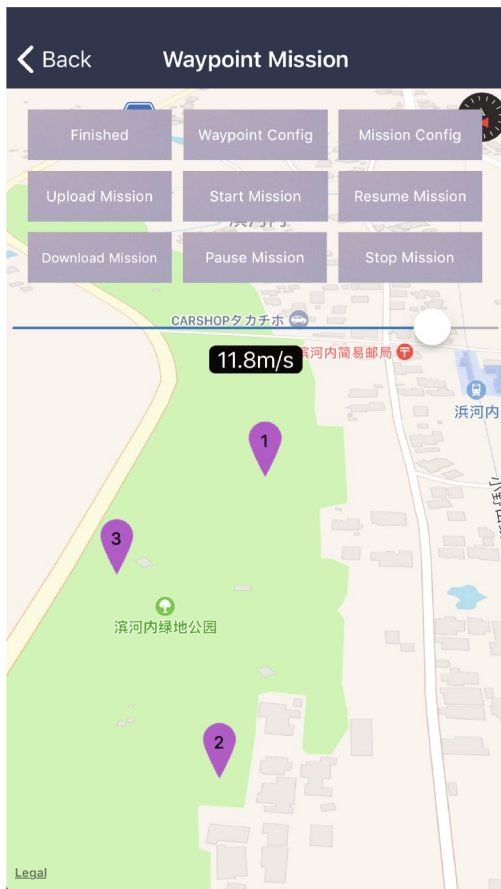
Fig. 11 An actual flight experiment could be successfully conducted using a mission plan
