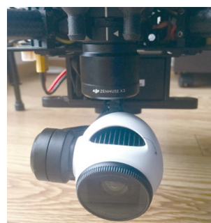
Fig. 8 Gimbal and RGB camera fixed under the quadrotor
