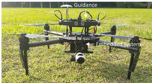
Fig. 3 Overview of the main body of the quadrotor with a guidance and an onboard embedded system
