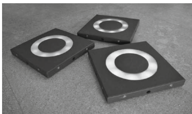
Fig. 2. The modular robotic tiles from Entertainment Robotics
