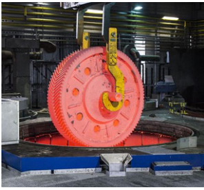
Fig. 1 Case hardening of large gears [8] as root-cause for changes in dimension and shape
