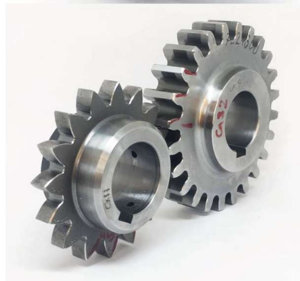
Fig. 6 Technical data of the FZG type A gear with internal cooling channels; pinion gear and gear pair
