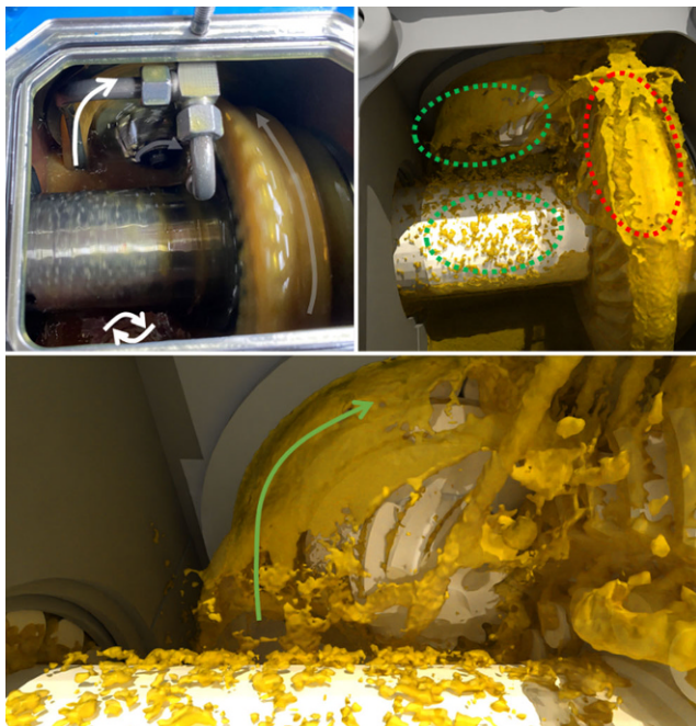
Fig. 5 Experimental ( left ) and simulation ( right ) flow field for a cold start OUT case at 600rpm
