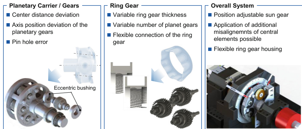
Fig. 3 Depicting elastic deformations at the test rig
