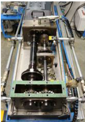
Fig. 4 FZG back-to-back test rig ( a = 91.5 mm) used for investigations of the tooth flank
