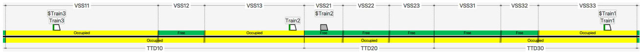
Fig. 6 Invalid system state: physical $Train2 is moving without sending a position report
