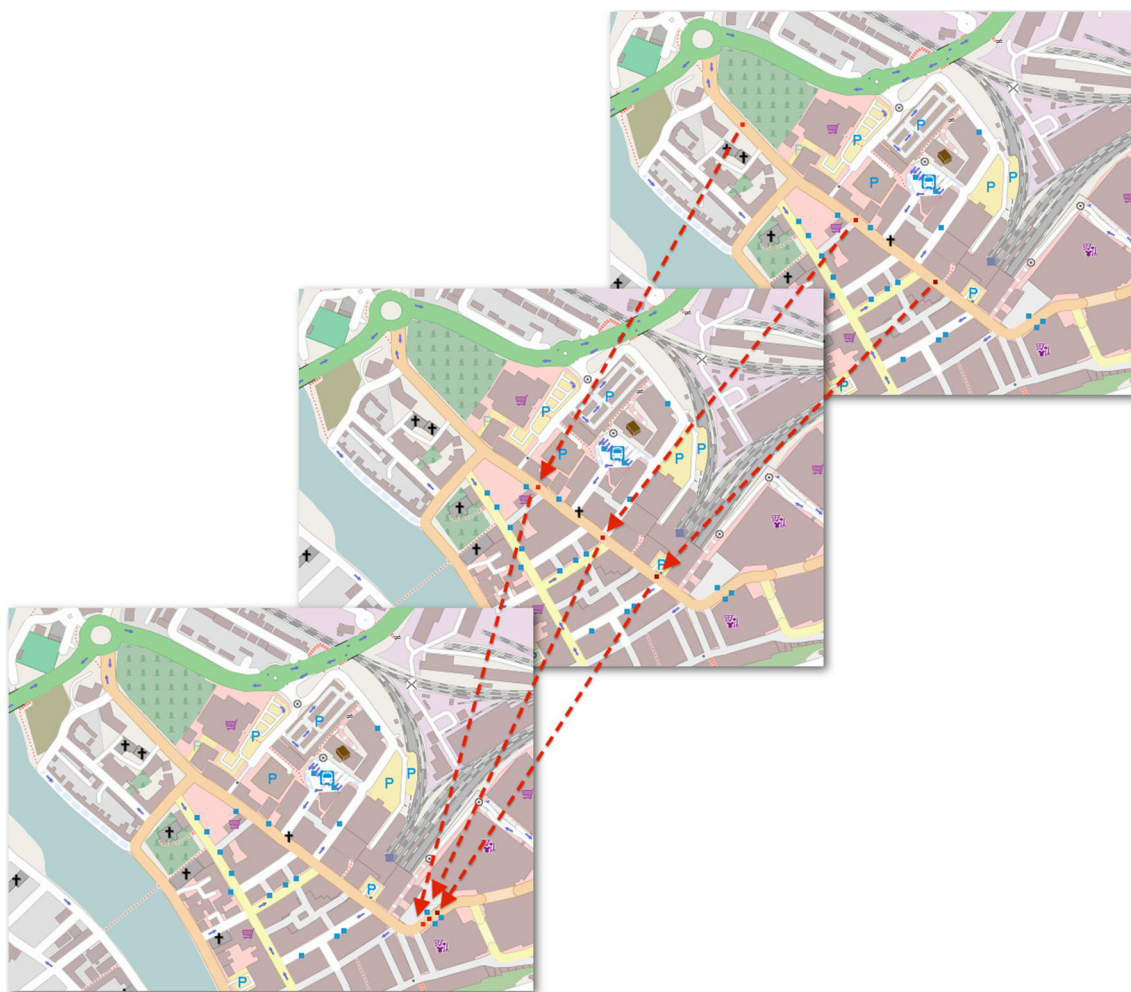
Fig. 9 Because of delays caused by boarding passengers, the headway between buses is successively eroded over time until the buses are essentially working as a conglomerate
