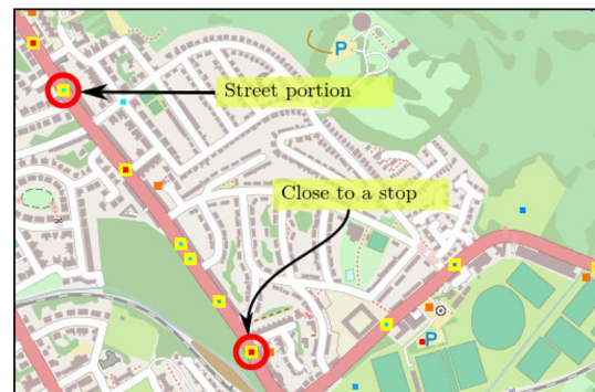
Fig. 5 Positions close to a stop are repainted in red, the areas of the road surrounding all bus positions are repainted in yellow (colour figure online)
