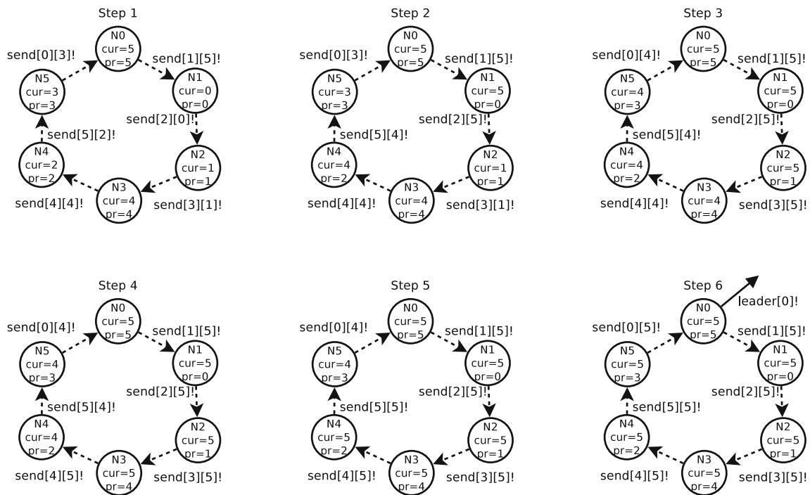
Fig. 6 Illustration of one scenario of how the information could be passed around the ring using the protocol. For the sake of illustration, every node happens to send the information to the next node at exactly
