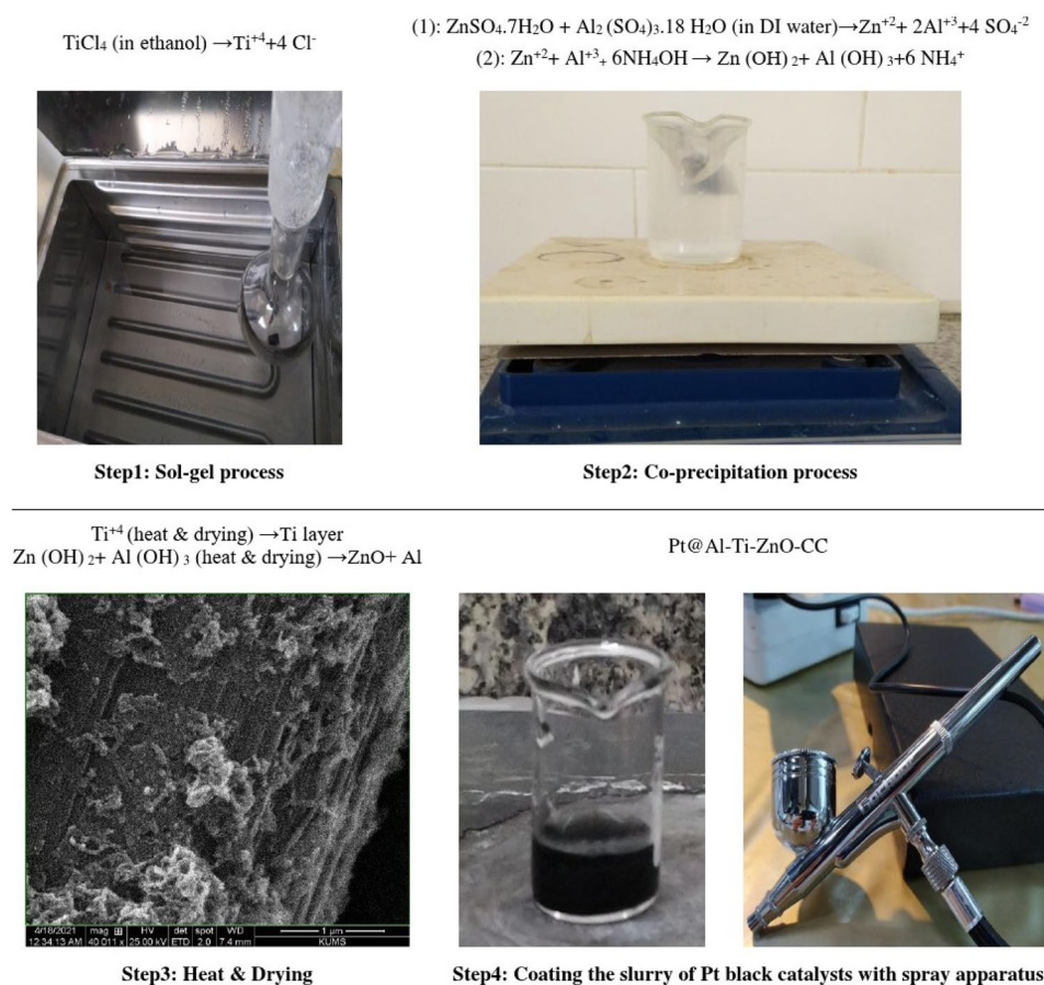
Fig. 1 The proposed reaction mechanism for the synthesis of catalyst supports
