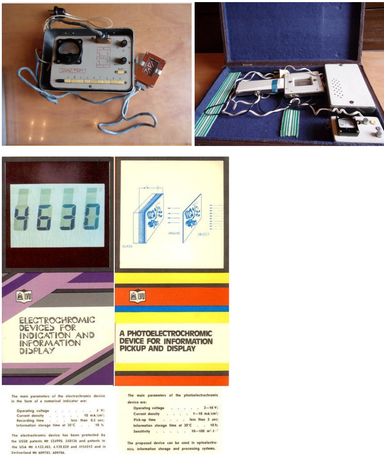
Fig. 1 Electrochromic and photo-electrochromic devices: prototypes and prospects (1980s)
