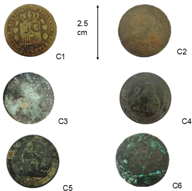
Fig. 1 The set of the studied ancient bronze coins showing a different degree of surface deterioration
