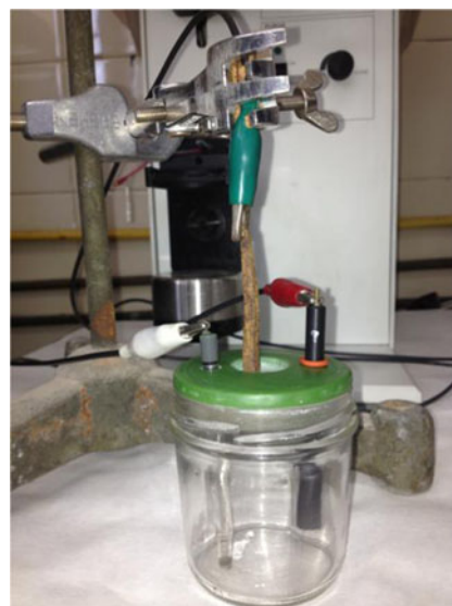
Fig. 1 Photographic image of the EIS cell with an iron nail from the Alcantarins convent (Ontinyent, Valencian Community, Spain) serving as a working electrode
