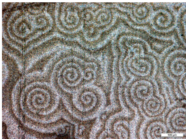
Fig. 5 Optical image of the In-Co alloy coating; 1 \text{ A dm}^{-2} , 62 wt.% Co, 3 \mu\text{m}
