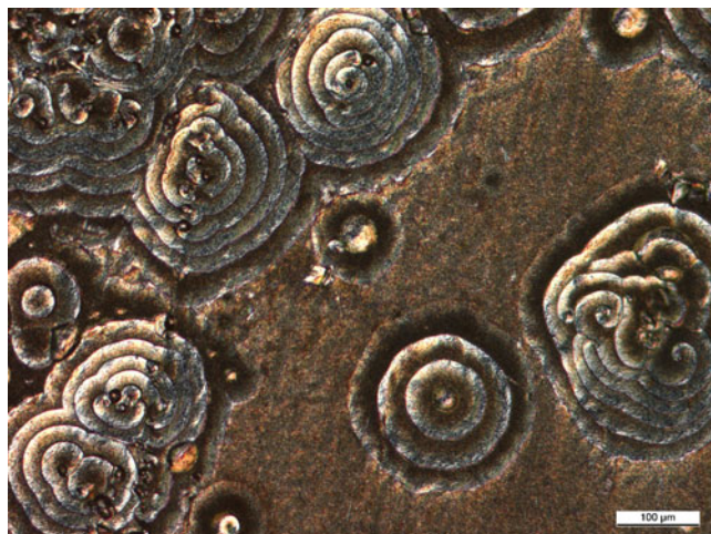
Fig. 3 Optical image of a Ag-Cd alloy coating; 1.2 \text{ Adm}^{-2} , 69 wt.% Cd, 9 \mu\text{m}
