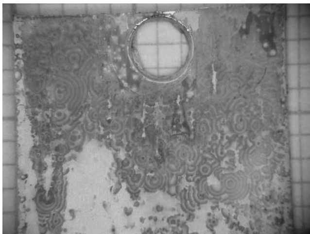
Fig. 8 Optical microscope image of a coatings surface before its detachment from the stainless steel substrate for X-ray measurement in the heating camera
