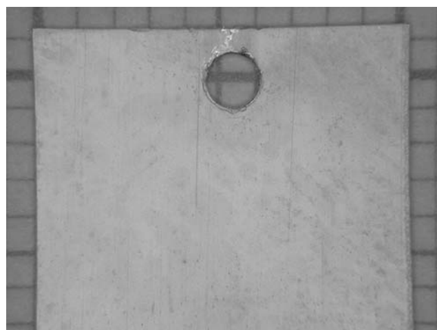
Fig. 2 Optical microscope image of the upper part of a coating deposited at 0.1 A dm -2 (electrode width – 1 cm, average In content less than 1 wt %)
