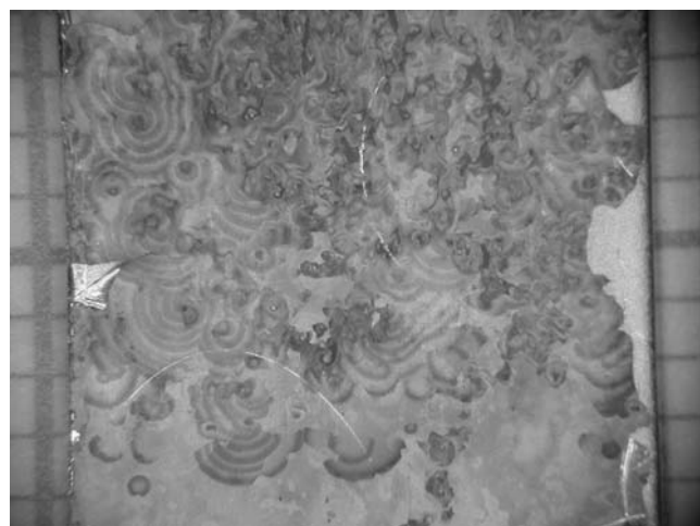
Fig. 7 Optical microscope image of a coatings surface before its detachment from the stainless steel substrate for DSC-measurement; c.d. – 0.15 \text{ A dm}^{-2} ; electrode width – 1 cm; average In content – 12.8 wt %
