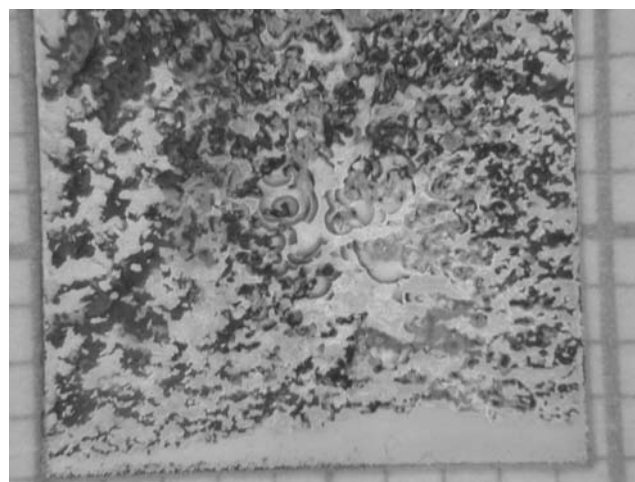
Fig. 4 Optical microscope image in the middle part of the surface of a coating; c.d. -0.5 \text{ A dm}^{-2} ; average In content 22.4 \text{ wt } \% ; electrode width -1 \text{ cm}
