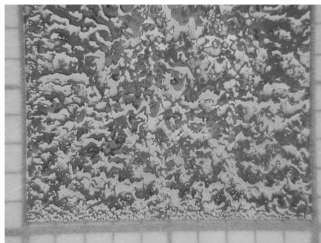
Fig. 5 Optical microscope image in the lower part of the surface of a coating; c.d. -0.9 \text{ A dm}^{-2} ; average In content 34.8 \text{ wt } \% ; electrode width -1 \text{ cm}
