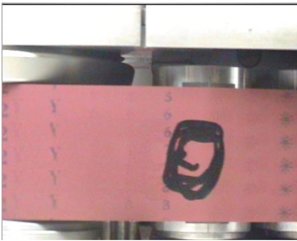
Fig. 4 Frame of a video recording of an open reel tape: the circle drawn in black marks a specific sound event. Often, in the electro-acoustic music field (in the works for tape and acoustic musical instruments) the marks on the tape are used as a synchronization means between live-electronics performer and the recorded tape music. If this information was not preserved, it would not be possible to perform the piece
