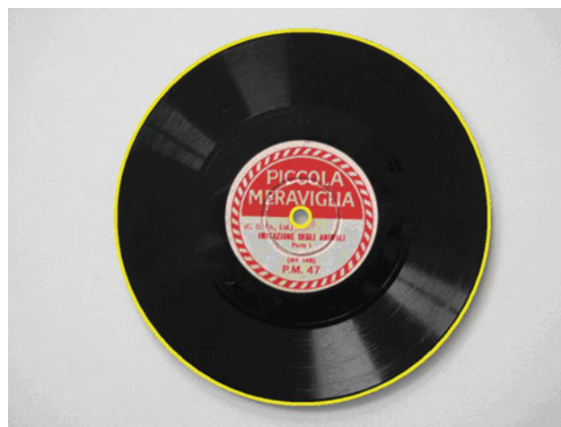
Fig. 9 Disk and spindle hole contours automatically detected via the integrodifferential operator
