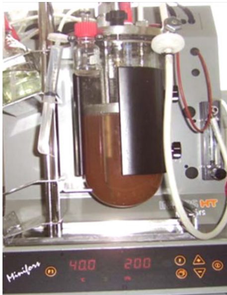
Fig. 1 The batch culture experimental setup used for the of biosurfactant production by the immobilized and free cells
