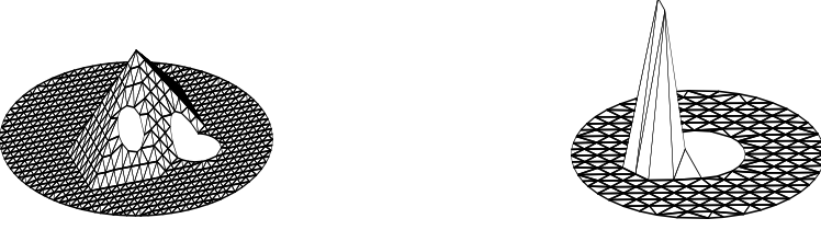
Fig. 3. Two typical basis functions of S_\ell^{CFE} . The shape of the basis functions is very similar to the standard hat functions where the support is restricted to the domain \Omega
