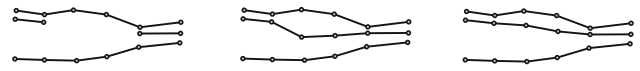
Fig. 4 Creation of smoothed height lookup tables \tilde{h}^l (2d slice). Left: initial height values. Edges to and between no-data values are not shown. Middle: no-data values are replaced through simple interpolation between upper/lower layer. Right: smoothing applied to new height values
