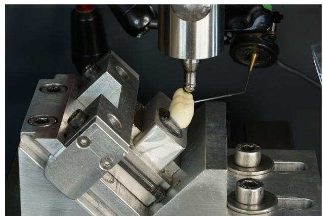
Fig. 4 Completely veneered zirconia CFPD in universal testing machine prepared for oblique loading with contact microphone attached
