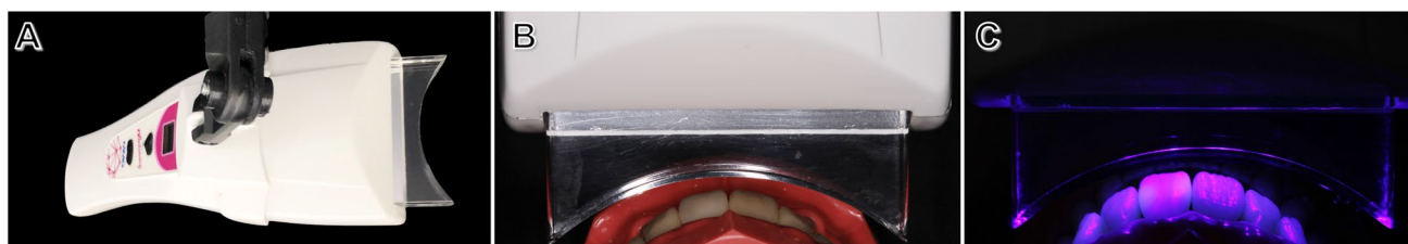
Fig. 2 Images of the V-LED light device: (A) the unit presents a curved acrylic tip coupled with the device's body. (B) The position of the light-emitting tip end held against the maxillary anterior arch of a dentiform model, note the manufacturer-recommended maximum
