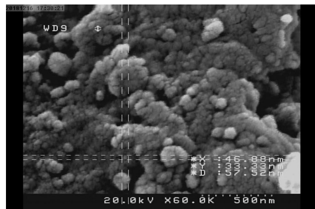
Fig. 1 A 6000 x view of the nanoparticle size of bioglass
