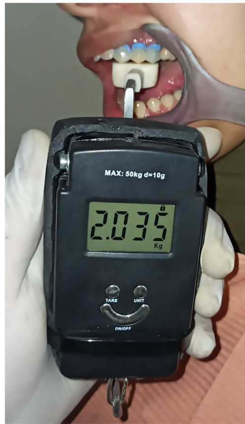
Fig. 1 Axial loading of the silicone light body with a modified tension gauge
