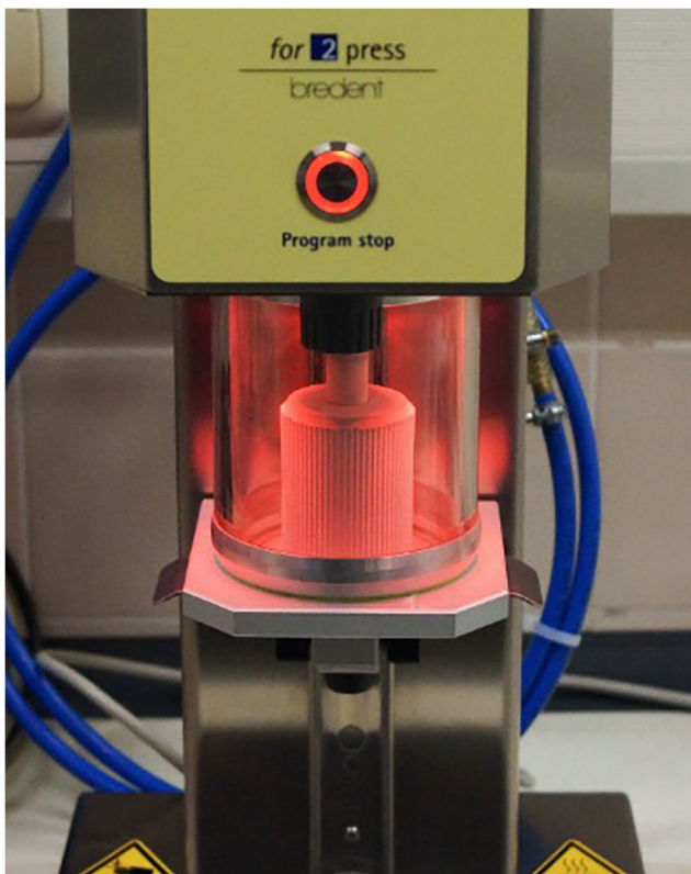
Fig. 3 Pressing process for clasps made from PEEKpressed (for 2 press, breident)
