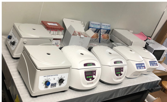
Fig. 2 Experimental setup: Each of the centrifuges were utilized in duplicate for a total of 6 centrifuges. From each patient, a total of 12 tubes were drawn (2 per machine) and centrifuged accordingly at either high- or low-speed protocol
