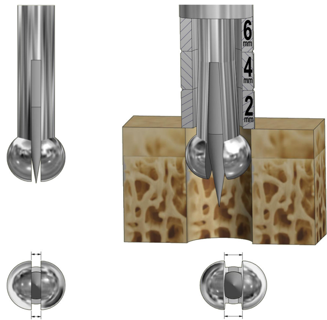
Fig. 2 Measurement principle of the precision instrument for diameter determination (Zentiness, Mahr). The instrument provides high precision measurement of diameter, roundness, and conicity of boreholes by spring-loaded halves of a measuring probe that is splitted by a protruding pin with a precision-lapped taper. This movement is transferred to an indicating instrument (not shown). (A) Neutral position of the measuring probe after calibration with a diameter ring gauge supplied by the manufacturer (not shown). (B) Expanded measuring probe during application on bone samples at the corresponding 2-, 4-, and 6-mm depths of the drilling hole
