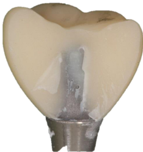
Fig. 4 Typical failure pattern after fracture test (example RIC)
