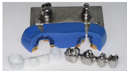
Fig. 1 Titanium basis model and frameworks (CoCr and zirconia) with replicas obtained per framework: four cross-sectional specimens (oro-vestibular and mesio-distal for both premolar and molar)
