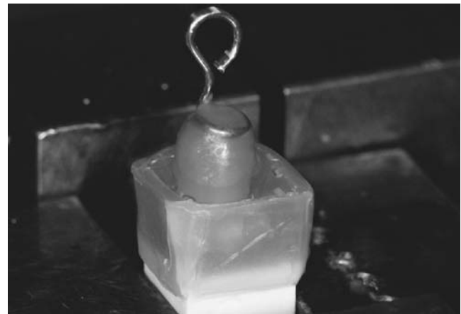
Fig. 3 Experimental setup: primary crown and electroformed coping set together for the separation process in the universal testing machine
