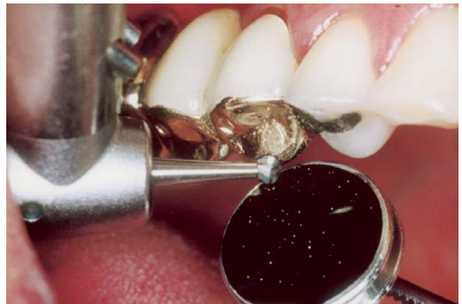
Fig. 2 Collection of grinding dust for alloy analysis
