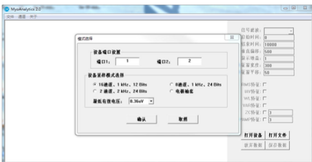
Fig. 2 Signal acquisition system interface
