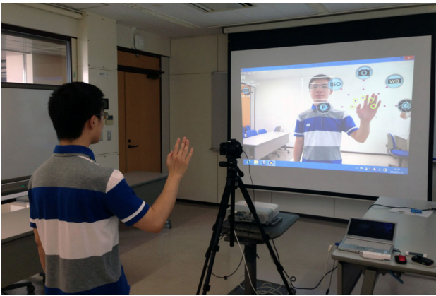
Fig. 1 The prototype system, which includes a DSLR camera, a projector, and a notebook PC. The user can use gestures to control the system to take self-portraits
