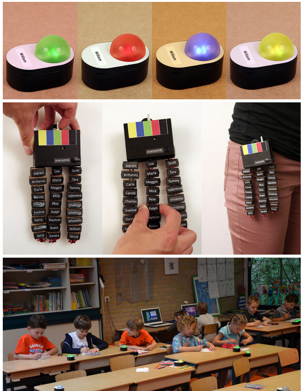
Fig. 3 Pictures of the FireFlies prototype: a light-object lit in different colors ( top ); the teacher-tool when selecting a color , selecting a child’s name and clipped to the user’s clothes; and FireFlies deployed in a primary school classroom
