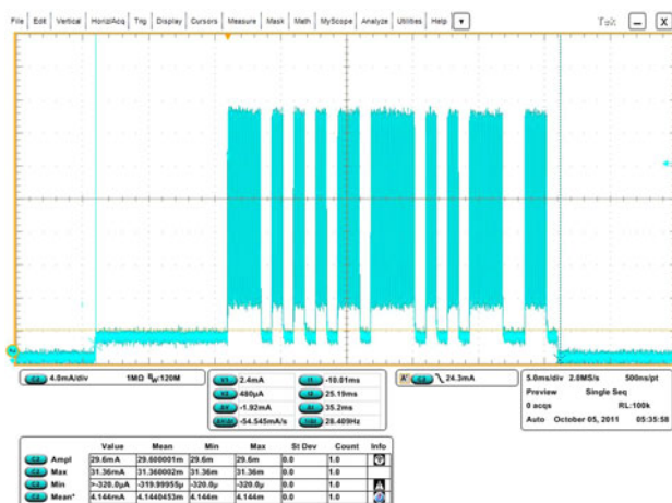
Fig. 12 Power analysis for the transmission of a drug identifier of 3 bytes carried out with the Tektronix DPO-7104C
