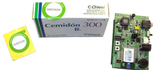
Fig. 4 Movital RFID module, with example of RFID tag and a box of drugs with RFID tag
