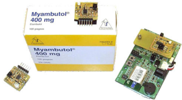
Fig. 5 Movital IrDA, with example of IrDA and box of drugs with IrDA-based tag
