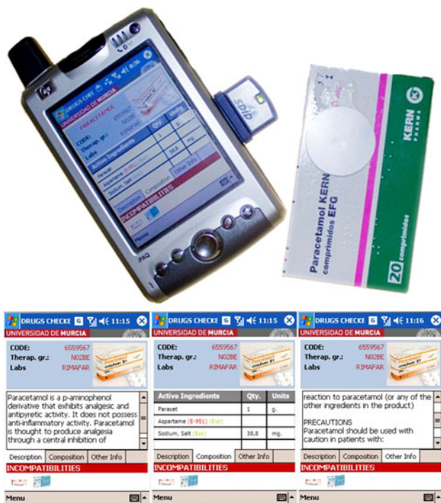
Fig. 11 Top : pocket PC with SDiD 1010 RFID card. Bottom : showing drug information and interactions
