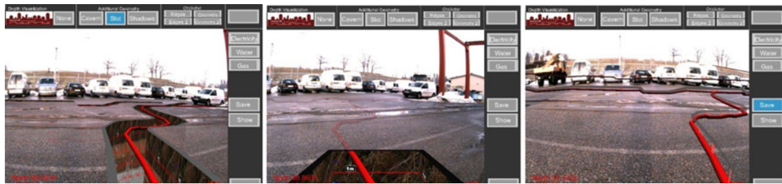
Fig. 7 Different visualizations of the same data of electricity lines. Left Simple blended overlay of a pipe using virtual ducts visualized along the pipes. Middle Advanced manhole visualization of a similar electricity pipe. Right Shadows of the pipes projected to the ground
