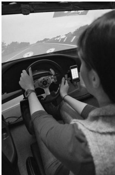
Fig. 2 The driving simulation setup (without the helmet-mounted eye-tracker). The mobile device was positioned on the right-hand side of the steering wheel. Head-Up-Display (HUD) meters for speed and rpm indicated the position of the vehicle on the lane
