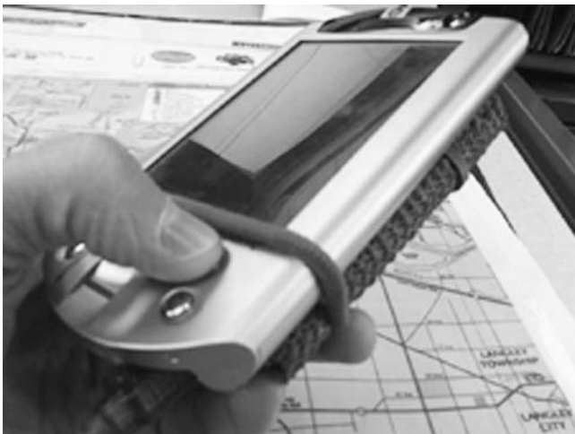
Fig. 4 Radio frequency identification reader attached to back of IPAQ handheld computer
