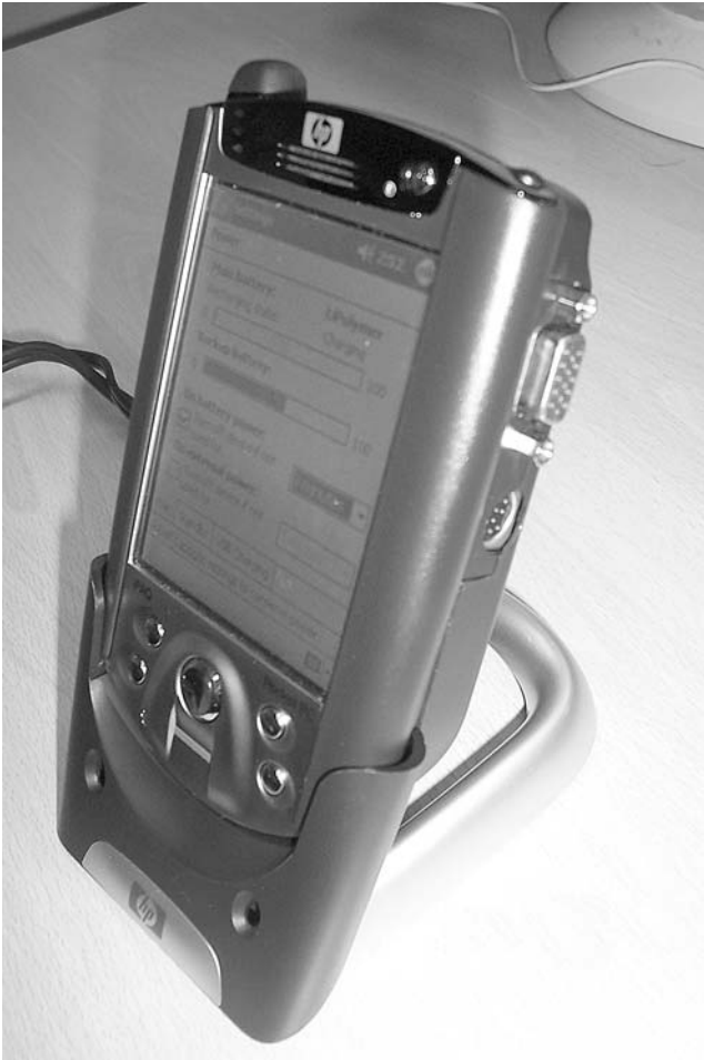
Fig. 2 Personal Digital Assistant with Lifeview Flyjacket i3800 attached
