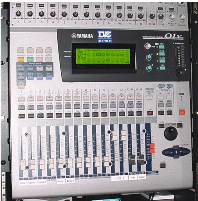
Fig. 2 In most electronic products, the controls clearly communicate the required actions (pushing, sliding, rotating etc.), but this does not necessarily mean that they communicate their function
