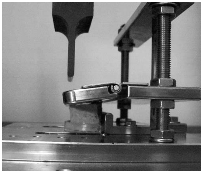
Fig. 1. Biomechanical testing. Each vertebra was compressed at a rate of 5 mm/min until the anterior height was decreased by 25%
