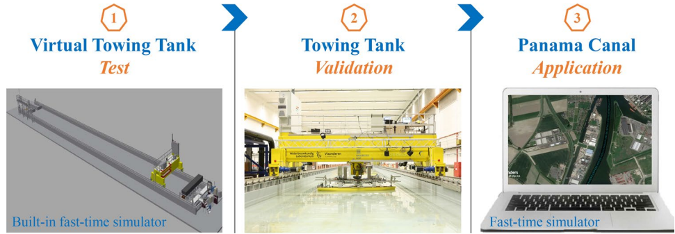
Fig. 12 Strategy of this research: (1) testing in the virtual towing tank built-in a fast time simulator; (2) validation in the towing tank; (3) applying in the simulator to run navigation simulations on Panama Canal
