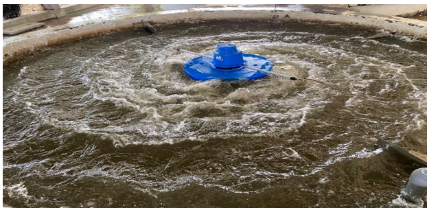
Fig. 10 Experimental round pool. The diameter of the round pool is 5 m and the depth is 1.5 m
