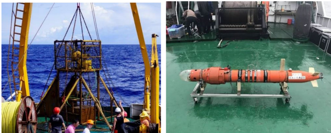
Fig. 16 The docking station and AUV in the sea trials (left: the dock; right: the AUV)
