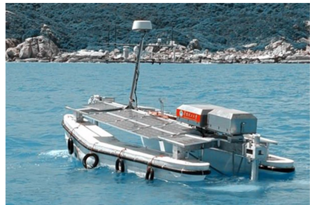
Fig. 2 The photograph of the unmanned catamaran ship completed driven by hydrofoils
