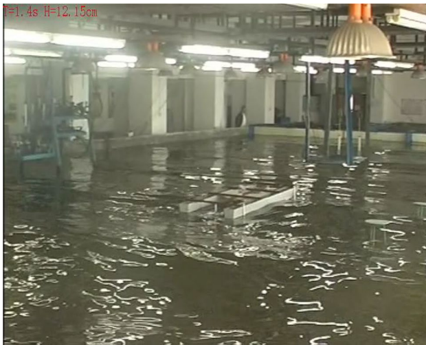
Fig. 11 Free running wave basin test of the catamaran model with passively pitch controlled foils
