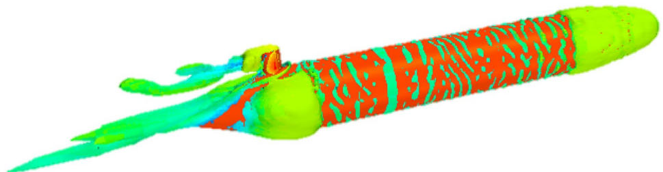
Fig. 7 Unsteady turbulent flow field of the SUBOFF model with appendage ( Q=10 )
